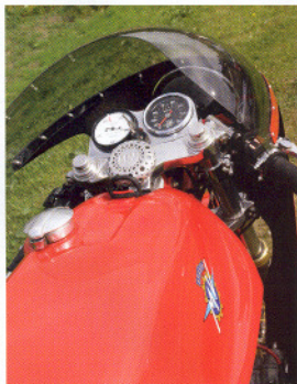
Above: Veglia instruments and beautifully machined MV steering damper knob complete the rider's view beyond the tank
