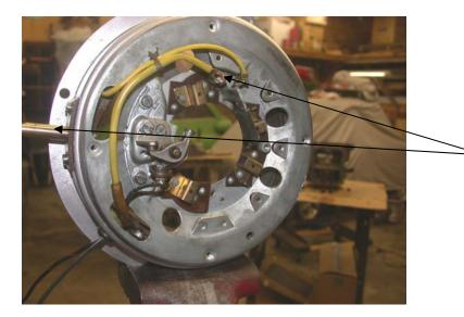
Connect the meter between the main post and the heavy yellow wire shown at the left. You should read close to "0" ohms.
