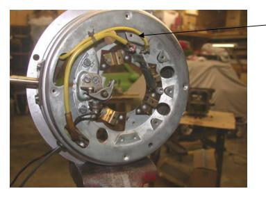
Connect the meter between this lead and the black / red lead in the dynastart wiring harness.
