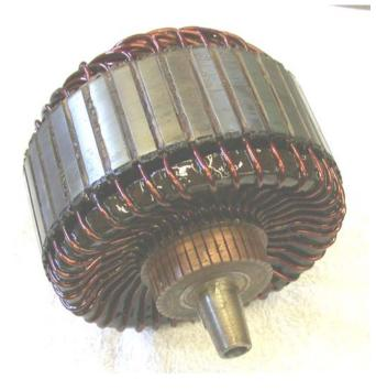
The field coil assembly is designed to carry both the series field and shunt fields. It also carries a set of points for the ignition system. The photo below does not show the points installed, but they would reside on the post shown in approximately the 1 o'clock position near the center hole. In addition, the larger brass post, with a nut on the top at about the 2 o-clock position, is the connection for the cable from the regulator
