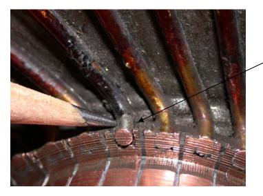
Solder joint was broken loose at this point and several other points on the commutator.
