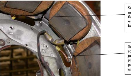
Solder joint between main post and the series field windings (starter windings). Check for loose solder joint.
