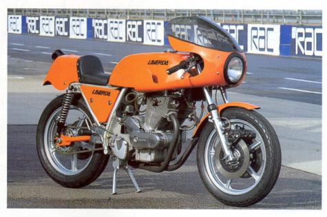
the standard 750 roadster. All engine components were specially selected, honed, heat treated and balanced to ensure maximum reliability rather than headline grabbing power figures. Which isn't to say it was slow. Each SFC engine had to make 70bhp at 7500rpm or it was back on the bench for more work
